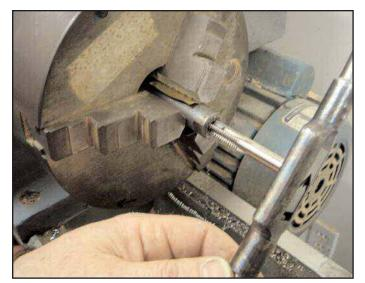
Figure 24. Tapping the shaft end.
